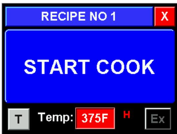
Once the operator has loaded the oven and advanced to this window they must touch the large button to start cooking.
