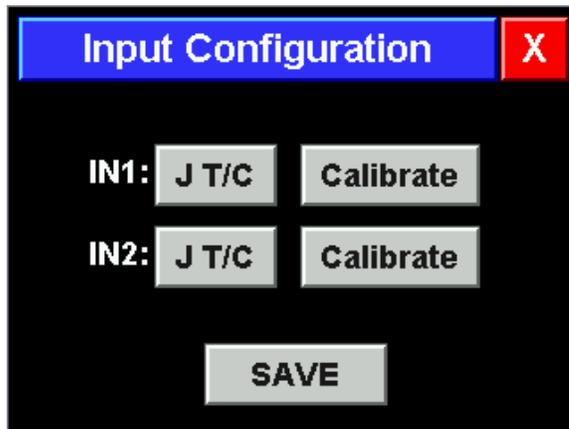
If you choose to re-calibrate either of the inputs you must have a thermocouple calibrator or precision 100 ohm and 200 ohm resistors, please contact Artisan for further information. The controller will lead the technician through a Zero and Gain calibration using the appropriate input value and recalibrate the sensor input. The thermocouple calibrator must supply a copper connection (not T/C metals) and have CJC compensation turned off for accurate calibration.
