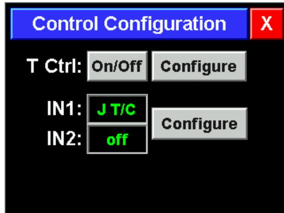
**T Ctrl:** Determines the method of temperature control and the configuration of that method. The control system always uses the first temperature input as the process variable. The button can be pressed to change from PID to ON/OFF control. The PID control output is always the SSR1 output, in ON/OFF control the output can be changed between K1 and SSR1 with an adjustable hysteresis value. The [Configure] button opens either the PID configuration window or the On/Off configuration window
