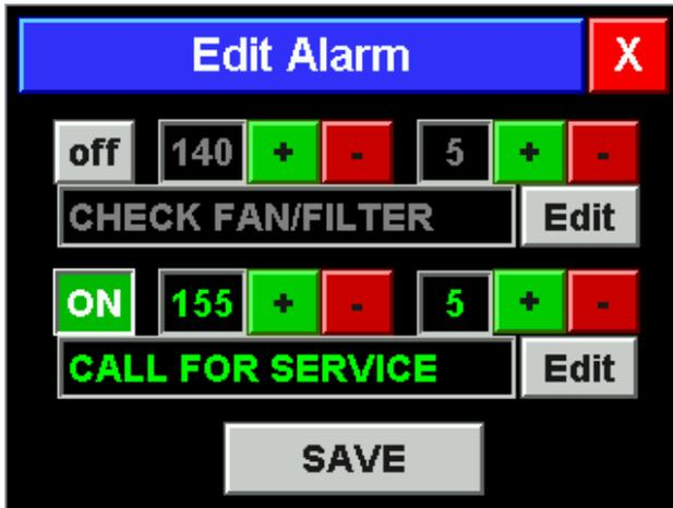
*NOTE: The upper CJ alarm temperature can be decreased as you choose but can not be increased above 155°F for the protection of the controller. In addition, this alarm can not be disabled like all of the other system alarms again for the protection of the controller.*
