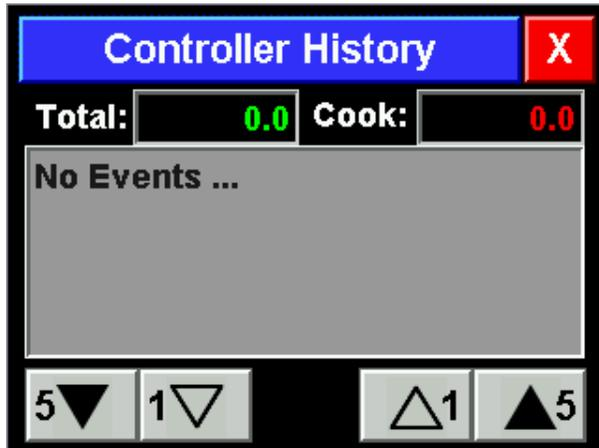
The scrollable list below the time values shows all of the trackable events and errors the controller has experienced, the controller remembers up the last 128 events. The date and time of the event and a descriptive string are displayed, use the up and down arrows to view the list.
