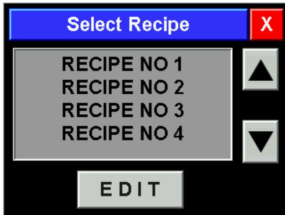
Press the [ Recipes] button in the configuration window and the Select Recipe window appears. Use the up and down arrows to scroll the recipe list until the desired recipe is shown. Touch the recipe to be edited and it is highlighted, then press the [E D I T] button and the recipe configuration is shown in the window and is ready for editing
