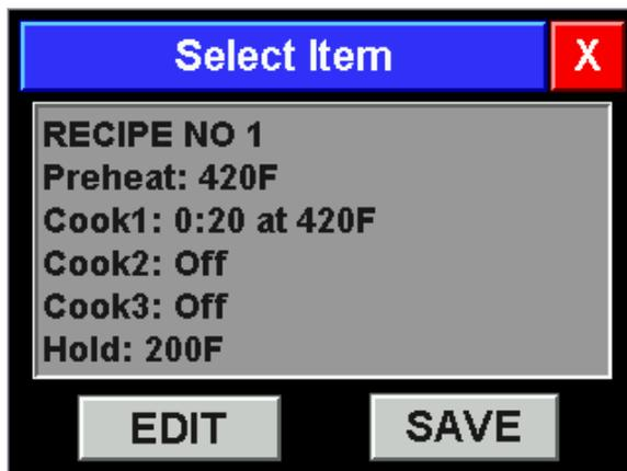
The number of cook and hold cycles displayed are dependent on the customization of the controller done by Artisan. The standard 5400 model has three different cook cycles and a hold cycle.
