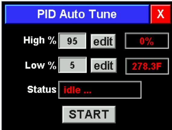
The High % value can be changed by pressing the [edit] button which displays a numeric entry window. The same method is used to edit the Low % value. The upper window on the right side displays the real-time output percentage and the window below is the temperature. The two percentage values are saved in the non-volatile memory with the other PID configuration information to simplify additional auto tuning cycles for maximum control tuning.
