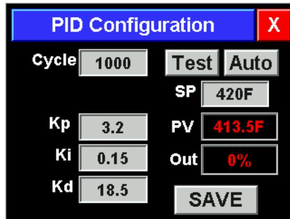
Cycle: This is the output cycling time and PID calculation cycle time in milliseconds, non-adjustable.
