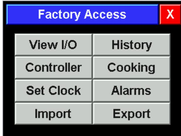
The [View I/O] button opens a window which shows the states of all inputs, allows the manual activation of all outputs, and from which the temperature offset from the probe to the visible temperature can be set.
