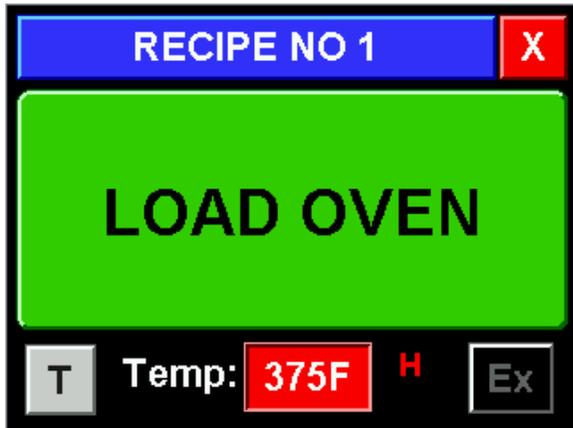
While this window is displayed the controller is monitoring the SW1 input. If the controller sees that the input changes state twice (indicating the door is opened and then closed) the controller advances to the START COOK window below. Alternately, the user may touch the large button.
