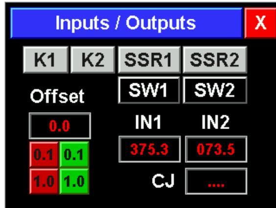
K1 & K2: These buttons change the state of the two relay contact outputs. Pressing one of these buttons will toggle its state (shown by a highlight change) and the state of the output relay.
